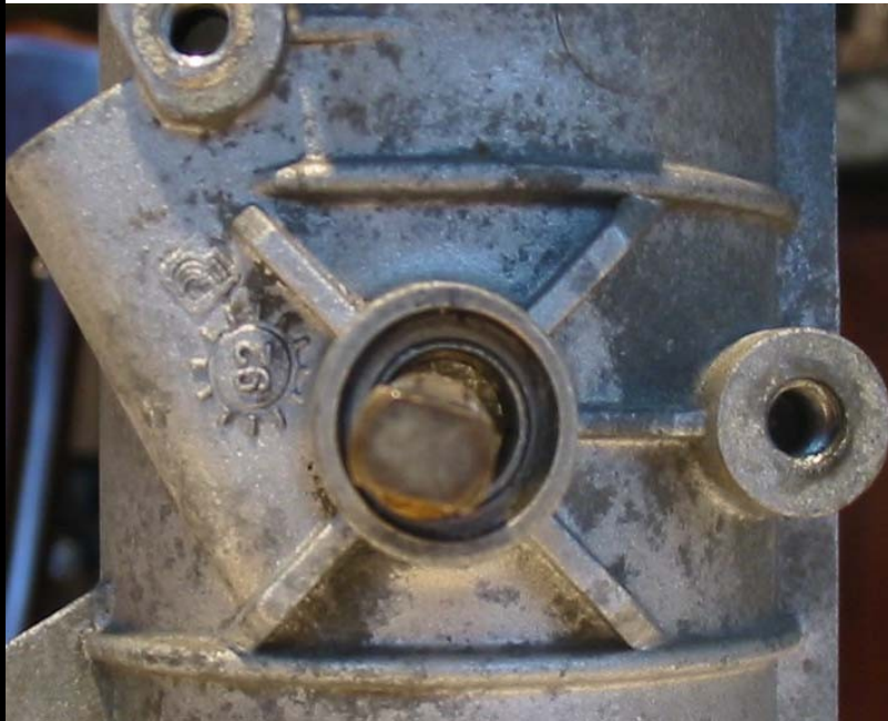
EXCESSIVE WEAR ON SHAFT SHOWN ON RIGHT SIDE
