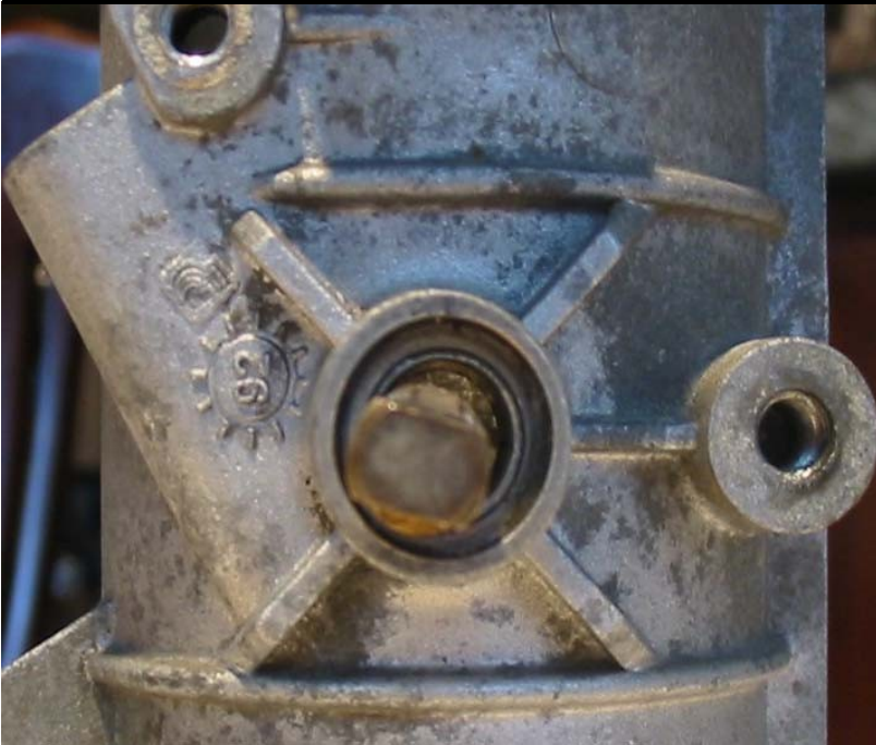
EXCESSIVE WEAR ON SHAFT SHOWN ON RIGHT SIDE
